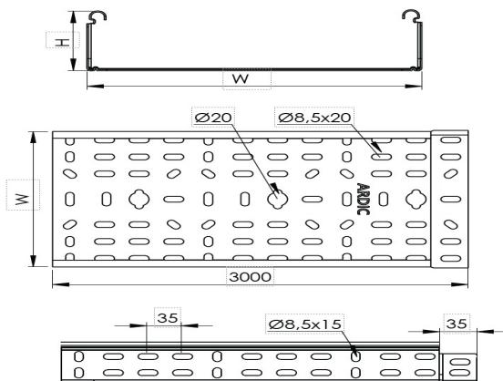
**ALL Cable Tray W150mm H60mm T1,5mm L:3000mm HDG****DIMENSIONS**
