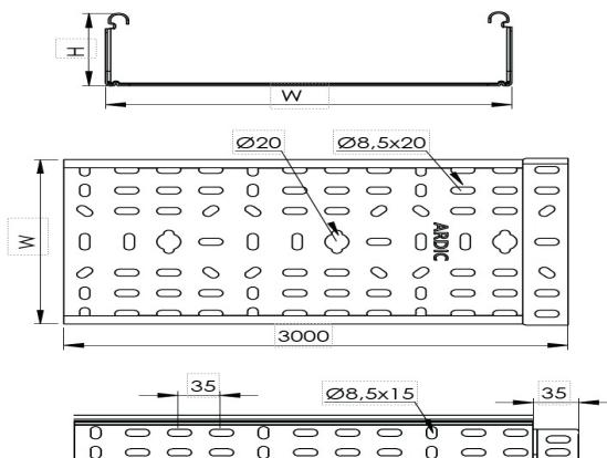
**ALL Cable Tray W300mm H60mm T1,2mm L:3000mm HDG****DIMENSIONS**
