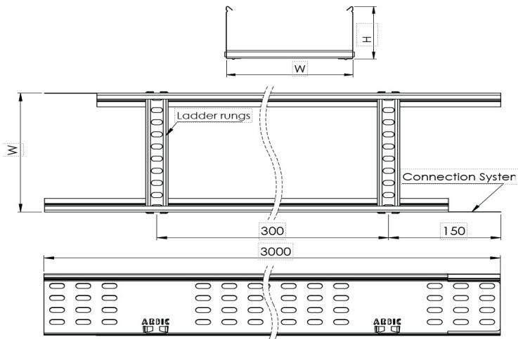
**CM Type Cable Ladder W150mm H40mm T1,5mm L:3000 HDG****DIMENSIONS**
