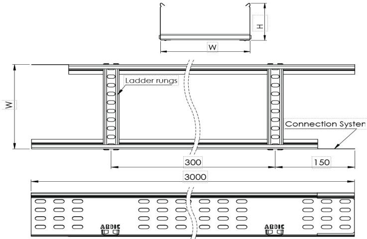
**CM Type Cable Ladder W200mm H40mm T1,5mm L:3000 PG****DIMENSIONS**
