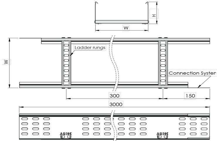
**CM Type Cable Ladder W300mm H40mm T1,5mm L:3000 PG****DIMENSIONS**
