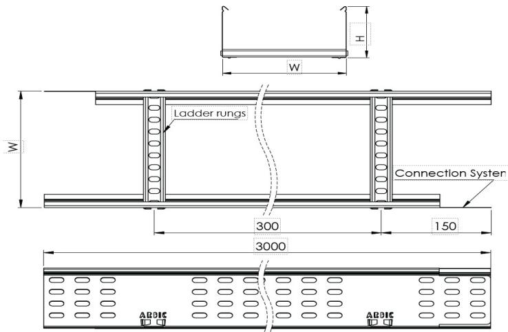
**CM Type Cable Ladder W300mm H40mm T1mm L:3000 PG****DIMENSIONS**
