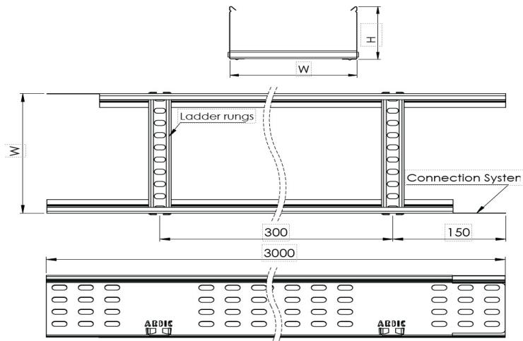
**CM Type Cable Ladder W400mm H40mm T1,2mm L:3000 PG****DIMENSIONS**
