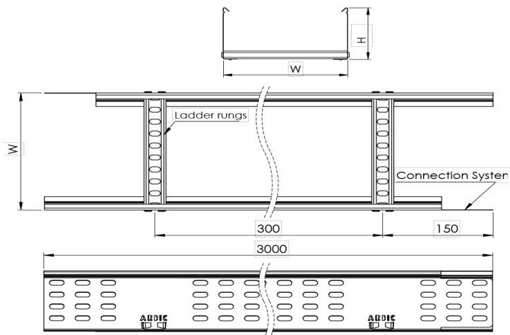
**CM Type Cable Ladder W600mm H40mm T1,2mm L:3000 PG****DIMENSIONS**
