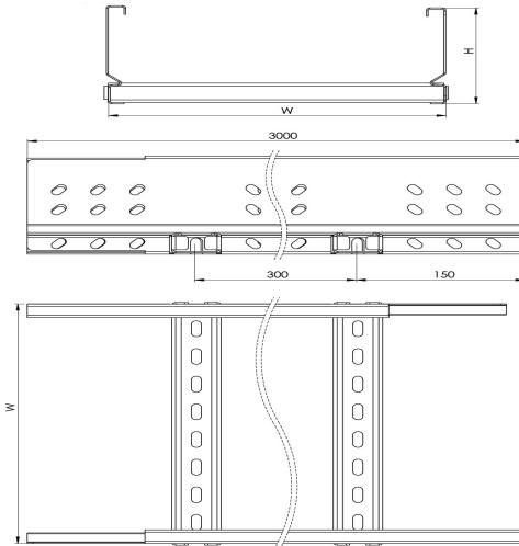
**FM Type Cable Ladder W150mm H125mm T1,5mm L:3000 PG****DIMENSIONS**
