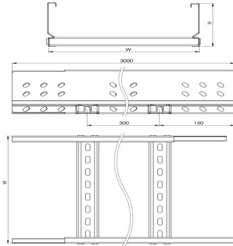
**FM Type Cable Ladder W150mm H125mm T2mm L:3000 HDG****DIMENSIONS**
