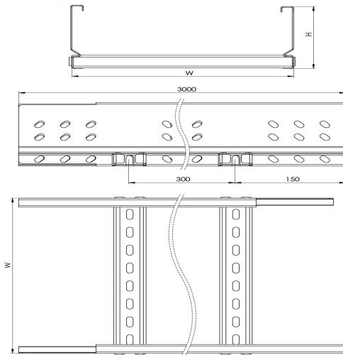
**FM Type Cable Ladder W800mm H150mm T1,5mm L:3000 HDG****DIMENSIONS**
