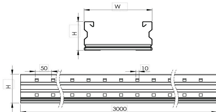
**FMD Type Cable Ladder W200mm H100mm T2mm L:3000mm PG****DIMENSIONS**
