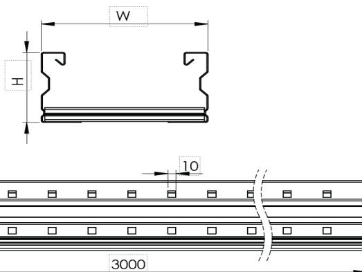
**FMD Type Cable Ladder W400mm H150mm T1,5mm L:3000mm PG****DIMENSIONS**
