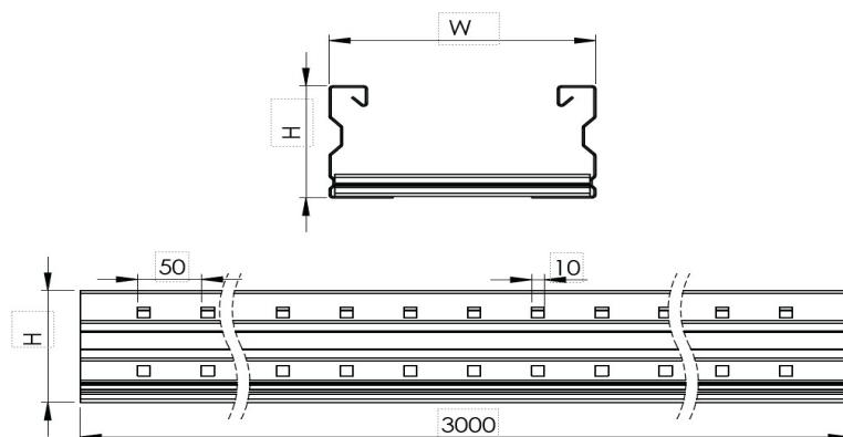
**FMD Type Cable Ladder W500mm H150mm T2mm L:3000mm HDG****DIMENSIONS**
