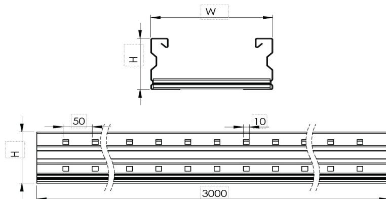
**FMD Type Cable Ladder W800mm H150mm T1,5mm L:3000mm PG****DIMENSIONS**
