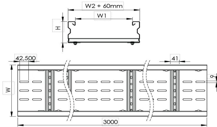
**FTD Cable Tray W300mm H100mm T2mm L:3000mm HDG****DIMENSIONS**
