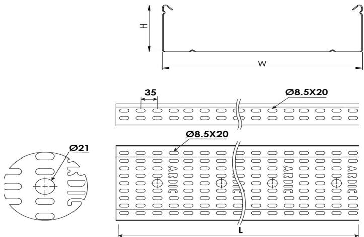
**Heavy Duty Cable Tray W1000mm H40mm T1,5mm L:3000 HDG****DIMENSIONS**
