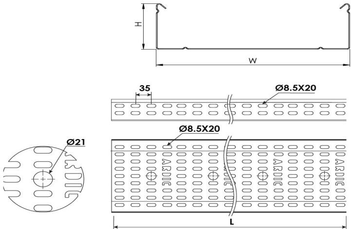
**Heavy Duty Cable Tray W100mm H50mm T0,8mm L:3000 HDG****DIMENSIONS**
