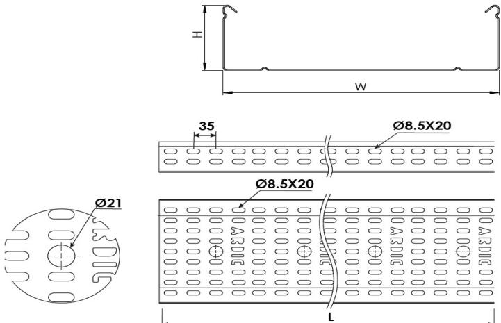
**Heavy Duty Cable Tray W100mm H50mm T0,8mm L:3000 PG****DIMENSIONS**
