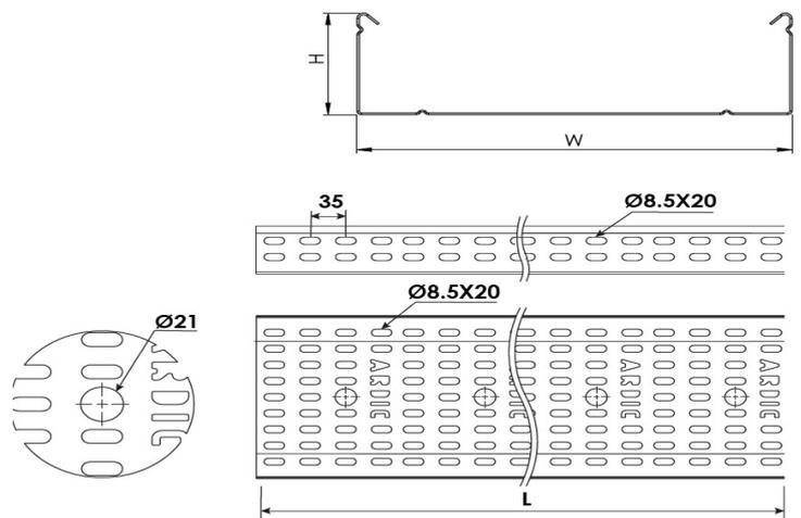
Heavy Duty Cable Tray W100mm H80mm T1,5mm L:3000 PG
