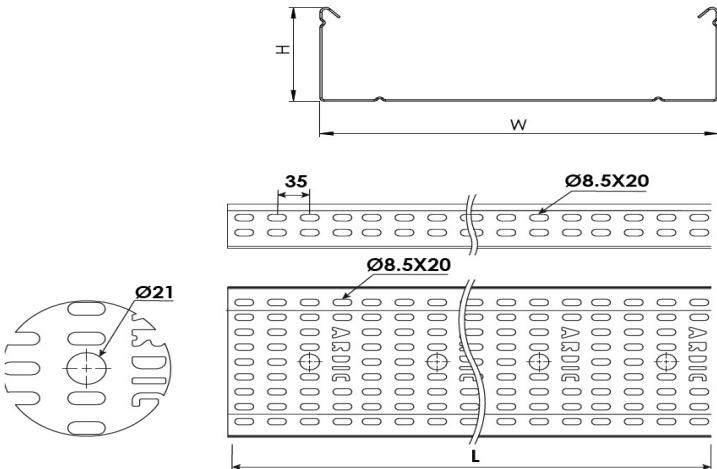
**Heavy Duty Cable Tray W100mm H80mm T2mm L:3000 PG****DIMENSIONS**
