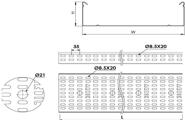
**Heavy Duty Cable Tray W150mm H50mm T0,8mm L:3000 PG****DIMENSIONS**
