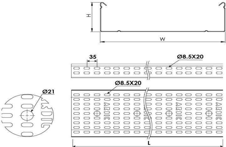
**Heavy Duty Cable Tray W150mm H80mm T2mm L:3000 HDG****DIMENSIONS**
