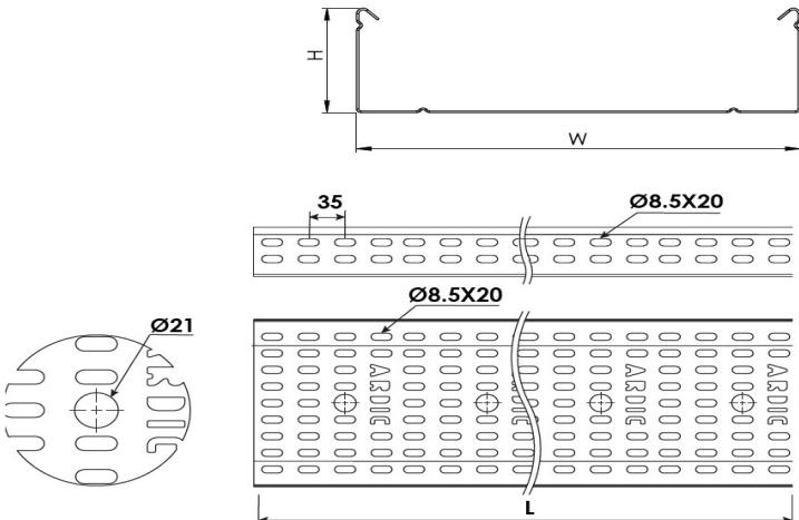
**Heavy Duty Cable Tray W250mm H80mm T1,5mm L:3000 HDG****DIMENSIONS**
