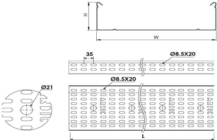
**Heavy Duty Cable Tray W400mm H80mm T1,5mm L:3000 PG****DIMENSIONS**
