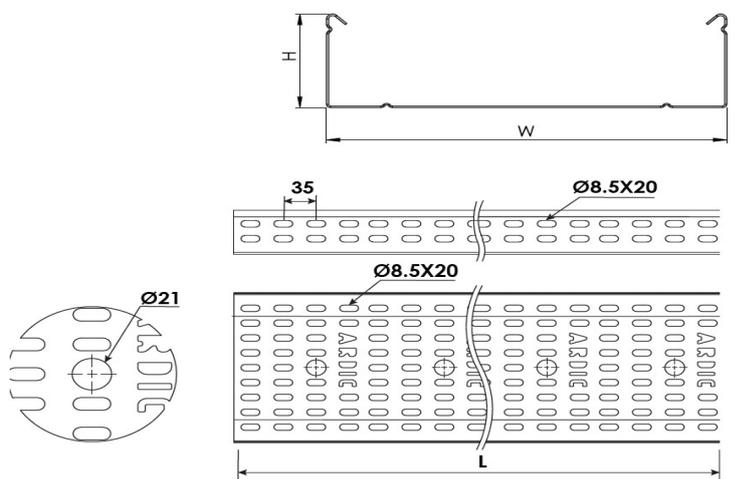
Heavy Duty Cable Tray W450mm H60mm T1mm L:3000 PG
