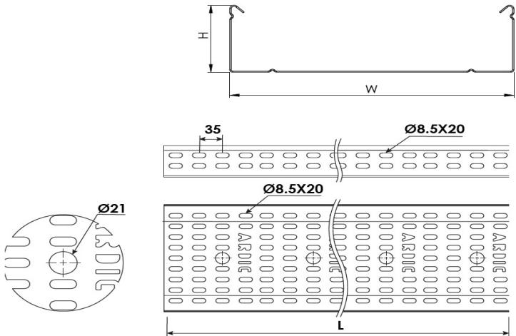
**Heavy Duty Cable Tray W450mm H80mm T2mm L:3000 HDG****DIMENSIONS**
