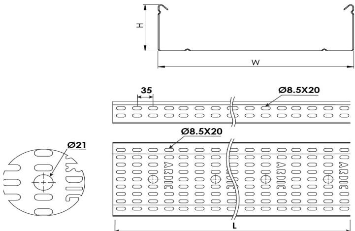
**Heavy Duty Cable Tray W700mm H50mm T1,5mm L:3000 HDG****DIMENSIONS**
