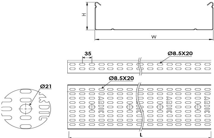
**Heavy Duty Cable Tray W800mm H80mm T2mm L:3000 PG****DIMENSIONS**
