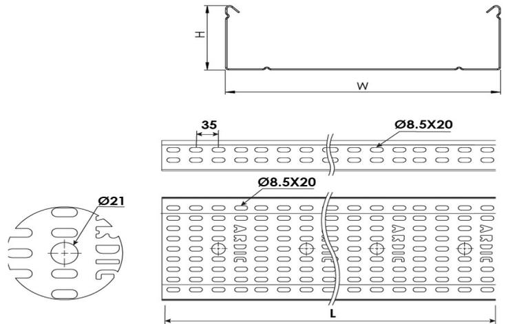
Heavy Duty Cable Tray W80mm H50mm T1,5mm L:3000 HDG
