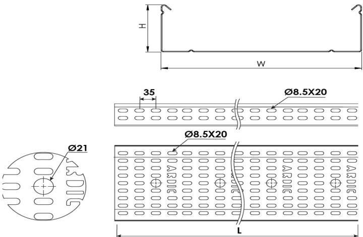
**Heavy Duty Cable Tray W900mm H100mm T1,5mm L:3000 PG****DIMENSIONS**
