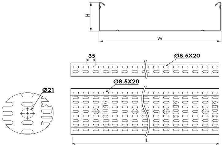
**Heavy Duty Cable Tray W900mm H40mm T2mm L:3000 PG****DIMENSIONS**
