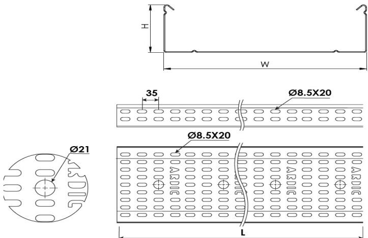
**Heavy Duty Cable Tray W900mm H60mm T1,5mm L:3000 HDG****DIMENSIONS**
