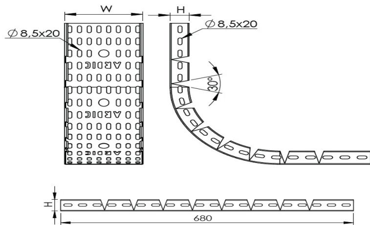
**İç-Dış Hareketli bükey W300mm H40mm T1,0mm PG****DIMENSIONS**
