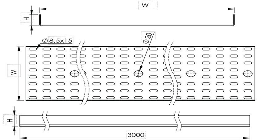
UK Cable Tray W450mm H15mm T2mm L:3000mm HDG
