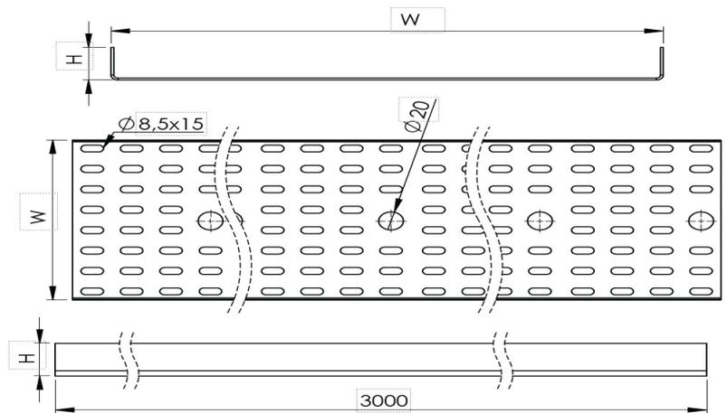
UK Cable Tray W50mm H25mm T1,2mm L:3000mm PG
