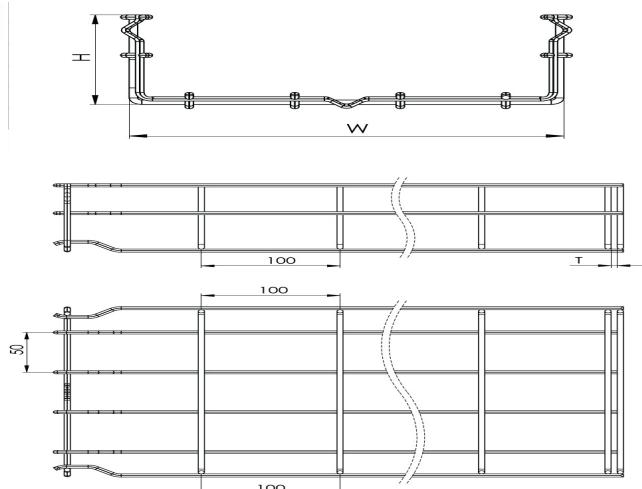
**Wire Mesh Cable Tray (Fast Connect Type) W200mm H100mm T4mm L:3000 HDG****DIMENSIONS**
