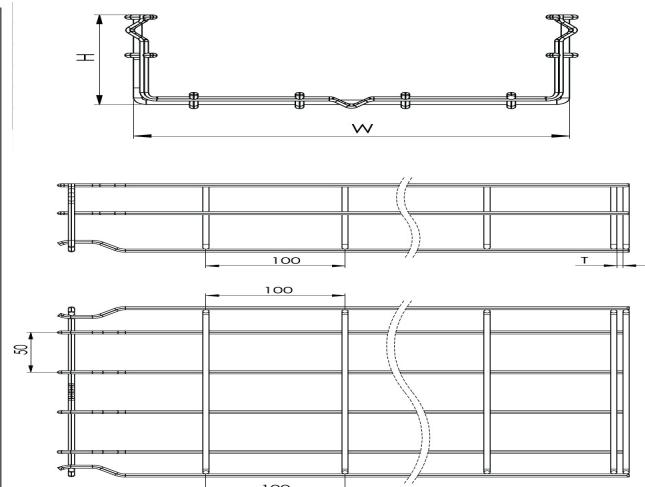
**Wire Mesh Cable Tray (Fast Connect Type) W250mm H35mm T4mm L:3000 HDG****DIMENSIONS**
