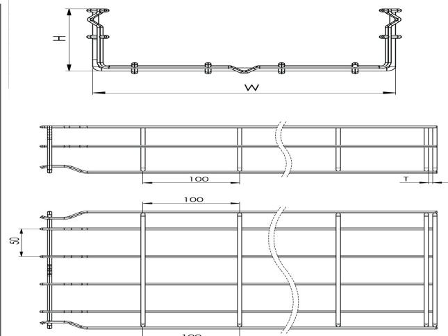
**Wire Mesh Cable Tray (Fast Connect Type) W250mm H35mm T5mm L:3000 EG****DIMENSIONS**
