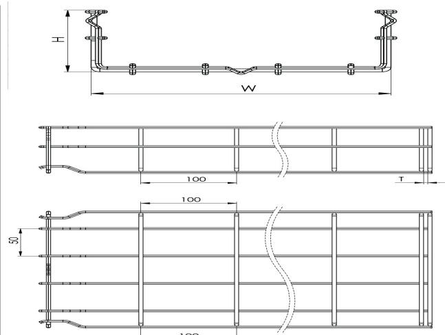
**Wire Mesh Cable Tray (Fast Connect Type) W250mm H35mm T5mm L:3000 HDG****DIMENSIONS**
