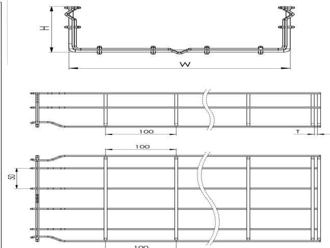
**Wire Mesh Cable Tray (Fast Connect Type) W300mm H100mm T4mm L:3000 HDG****DIMENSIONS**
