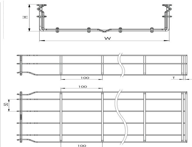
**Wire Mesh Cable Tray (Fast Connect Type) W350mm H35mm T4mm L:3000 SS304****DIMENSIONS**
