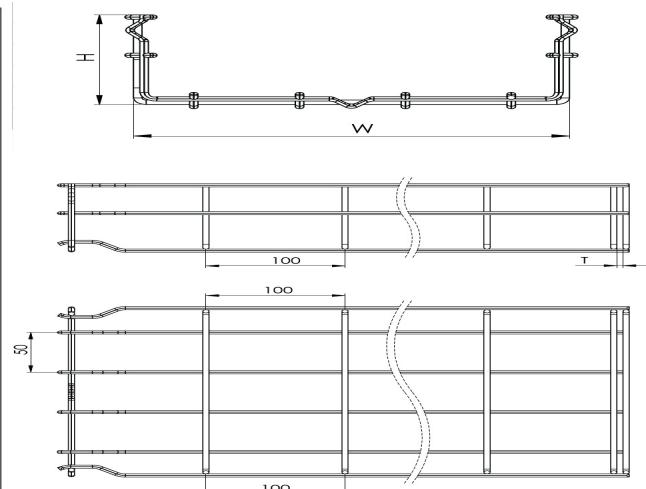
**Wire Mesh Cable Tray (Fast Connect Type) W400mm H35mm T4mm L:3000 SS304****DIMENSIONS**
