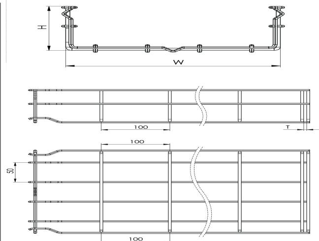
**Wire Mesh Cable Tray (Fast Connect Type) W400mm H35mm T5mm L:3000 SS304****DIMENSIONS**
