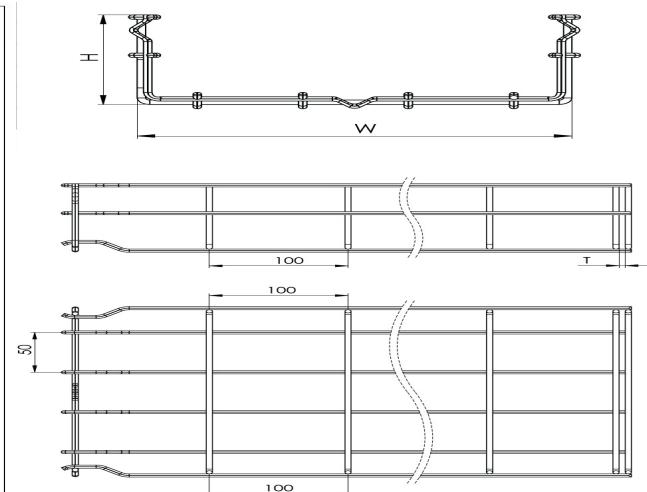
**Wire Mesh Cable Tray (Fast Connect Type) W450mm H100mm T4mm L:3000 SS304****DIMENSIONS**
