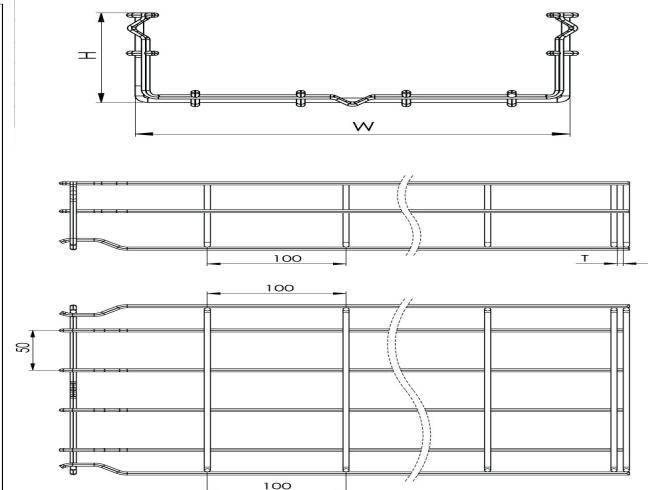
**Wire Mesh Cable Tray (Fast Connect Type) W450mm H100mm T5mm L:3000 SS304****DIMENSIONS**
