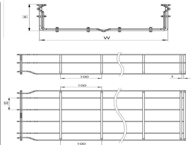
**Wire Mesh Cable Tray (Fast Connect Type) W450mm H35mm T4mm L:3000 SS304****DIMENSIONS**
