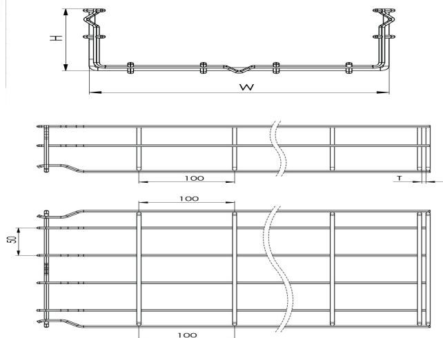
**Wire Mesh Cable Tray (Fast Connect Type) W500mm H100mm T5mm L:3000 SS304****DIMENSIONS**
