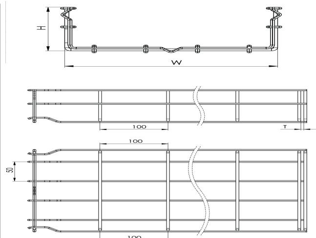
**Wire Mesh Cable Tray (Fast Connect Type) W500mm H35mm T5mm L:3000 SS304****DIMENSIONS**
