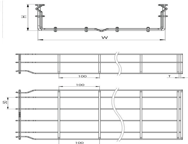
**Wire Mesh Cable Tray (Fast Connect Type) W550mm H100mm T4mm L:3000 SS304****DIMENSIONS**
